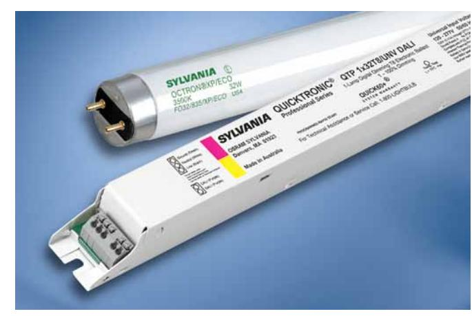
QUICKTRONIC DALI T8 Dimming ballasts offers full rated lamp output (1.0 ballast factor) at the maximum light setting. Compared to "normal" systems (0.88 ballast factor), this allows for higher light levels when desired and can be used to compensate for lamp lumen depreciation.
